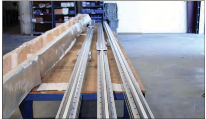
Bishop-Wisecarver specializes in long length challenges. Belt and chain driven LoPro linear actuators have been fabricated up to 80 feet.
