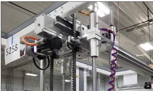
In the food product packaging industry, a LoPro system provides long overhead actuation for an automated material transfer system.
