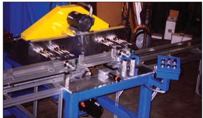
LoPro's precise travel and fast acceleration allow exact and repeatable hole drilling for door manufacturing, despite the presence of carbon fiber debris.
